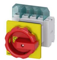
SENTRON, Switch disconnector 3LD, emergency switching-off switch, 4-pole, lu: 25 A, operating power / at AC-23 A 400 V: 9.5 kW, front-mounted, 1 NC, 1 NO, rotary operating mechanism, Red / yellow, Central mounting 22.5 mm of the handle
