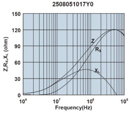
Impedance, reactance, and resistance vs. frequency.
