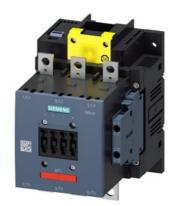
Power contactor, AC-3 185 A, 90 kW / 400 V Coil AC 50/60 Hz and DC 96-127 V x (0.8-1.1) F-SPS input 24 V DC 3-pole size S6 Auxiliary contacts 2 NO + 2 NC permanently mounted Main circuit: Busbar Control and auxiliary circuit: Screw terminal
