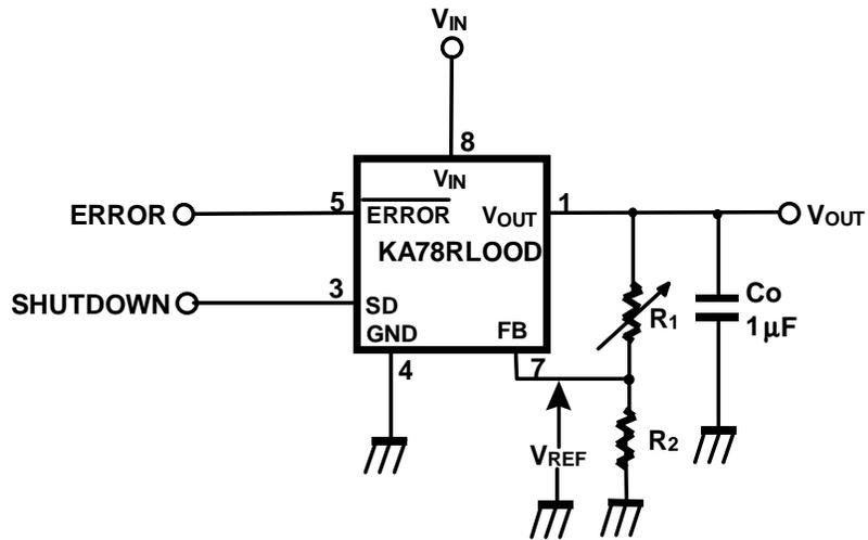
$$V_O = V_{REF} (1 + R_1 / R_2) + I_{FB} R_1$$
