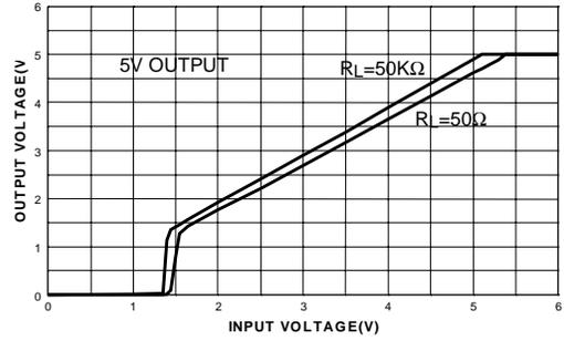
Figure 2. Dropout Characteristics
