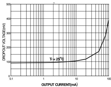
Figure 8. Dropout Voltage
