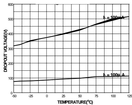
Figure 7. Dropout Voltage
