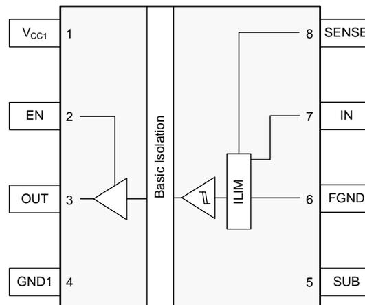
Figure 1. ISO1211 Isolated Digital-Input Receiver Pin Configuration
