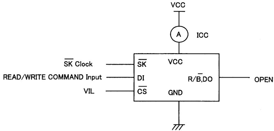
Fig-8 Operating Current test circuit
