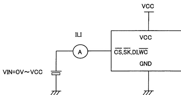
Fig.-6 Input leakage current test circuit
