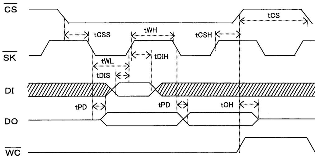
Fig.-10 Synchronous data input output timing
