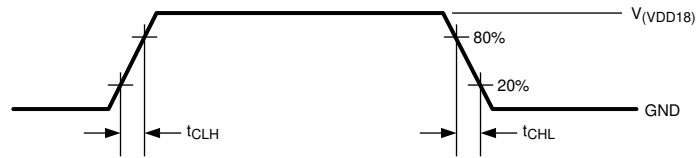
Figure 6-1. LVC MOS Transition Times
