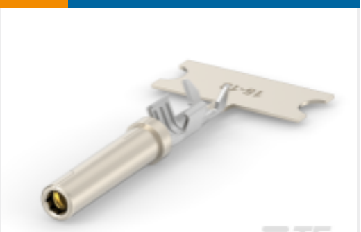
TE Part #3-2600021-5 XRC SOCKET 14-18 AWG Gold Plated
