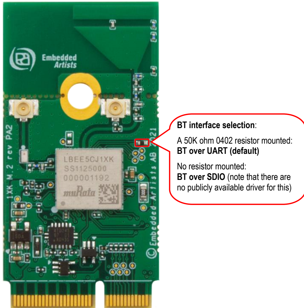
Figure 5 – 1XK M.2 Module Bluetooth Interface Selector
