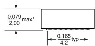
\* For optional tin-lead and silver-copper terminations, dimensions are for the mounted part. Dimensions before mounting can be an additional 0.005 inch / 0.13 mm.
