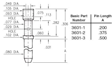
Description: 3601 - Wire Crimp Pin Packaging: Packaged in Bulk
