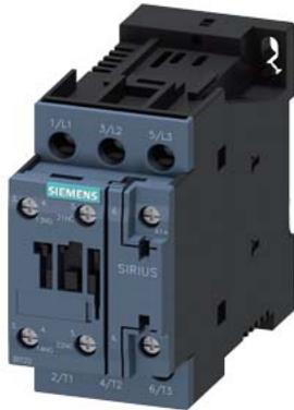
power contactor, AC-3e/AC-3, 12 A, 5.5 kW / 400 V, 3-pole, 60 V DC, auxiliary contacts: 1 NO + 1 NC, screw terminal, size: S0
