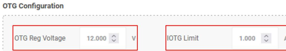
**Figure 2-10. OTG Configuration Section**
