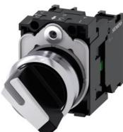
Selector switch, illuminable, 22 mm, round, metal, shiny, white, selector switch, short, 2 switch positions O-I, latching, actuating angle  $90^{\circ}$ , 10:30h/13:30h, with holder, 1 NO, 1 NC, screw terminal
