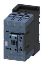
power contactor, AC-3e/AC-3, 80 A, 37 kW / 400 V, 3-pole, 110 V AC, 50 Hz, auxiliary contacts: 1 NO + 1 NC, screw terminal, size: S3  $\,$
