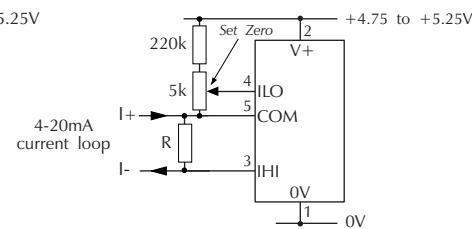
Measuring a 4-20mA loop current.
