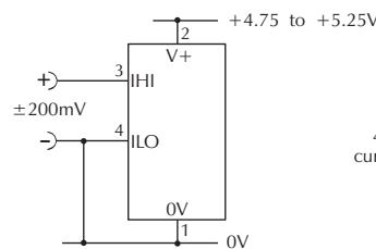
Measuring a single ended input voltage referenced to supply, i.e. the input voltage and the meter's power supply share the same 0V rail.
