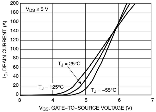
Figure 2. Transfer Characteristics
