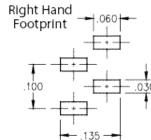
**Description:** Interconnect Socket .050 Grid; Surface Mount Socket Single Row Gull Wing; Right Hand Footprint Single Row Surface Mount Plating Code: 43
