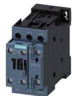
power contactor, AC-3e/AC-3, 32 A, 15 kW / 400 V, 3-pole, 48 V DC, auxiliary contacts: 1 NO + 1 NC, screw terminal, size: S0
