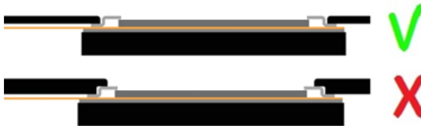
Figure 19. Positioning of the sensor
