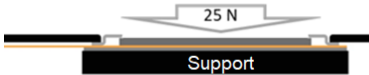
Figure 20. Integration shall withstand a pressure of at least 25N
