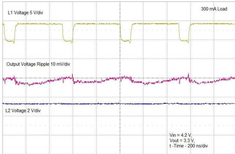
Figure 4. Output Ripple Vin 4.2 V
