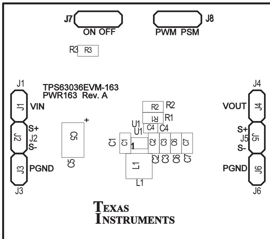
Figure 6. Assembly Layer
