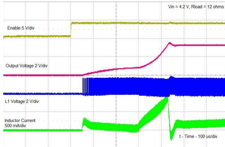
**Figure 2. Turn ON into Load,  $V_{in} = 4.2\text{ V}$**
