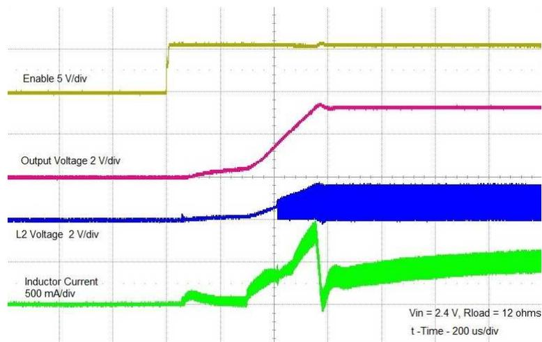
**Figure 1. Turn ON into Load,  $V_{in} = 2.4\text{ V}$**
