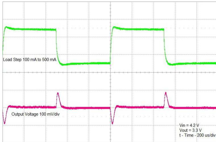
Figure 5. Load Step 100 mA to 500 mA
