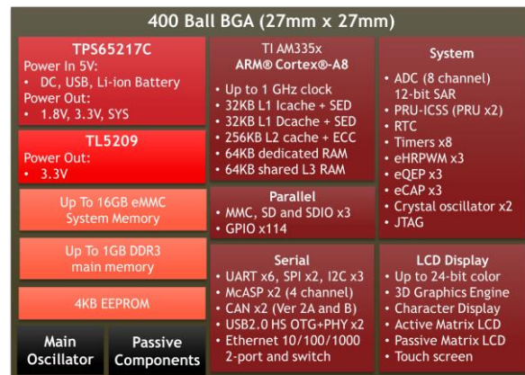
OSD335x C-SiP Block Diagram
