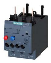
Overload relay 3.5...5.0 A Thermal For motor protection Size S0, Class 10 Contactor mounting Main circuit: Screw Auxiliary circuit: Screw Manual-Automatic-Reset
