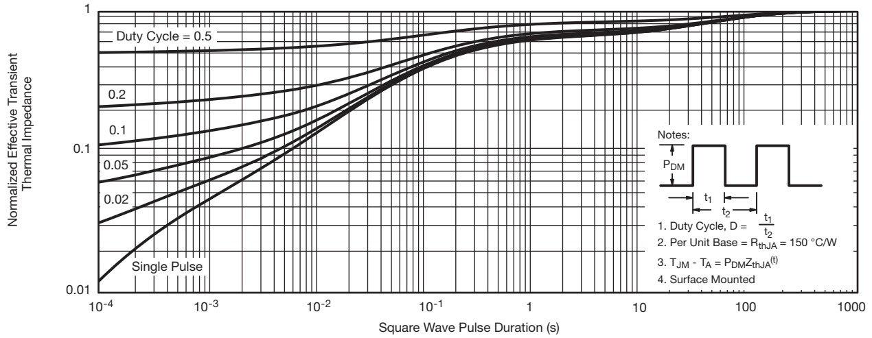
Normalized Thermal Transient Impedance, Junction-to-Ambient
