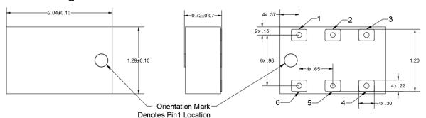
Configuration 1 Configuration 2 Configuration 3 Configuration 4 Pin Input Isolated Direct Coupled 2 GND GND GND GND Isolated Coupled 3 Input Direct Coupled Input 4 Direct Isolated 5 GND GND GND GND 6 Coupled Direct Isolated Input
