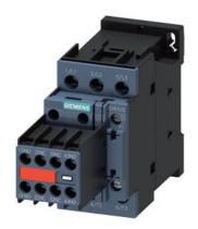
power contactor, AC-3e/AC-3, 32 A, 15 kW / 400 V, 3-pole, 230 V AC, 50/60 Hz, with plugged-in varistor, auxiliary contacts: 2 NO + 2 NC, screw terminal, size: S0, captive auxiliary switch
