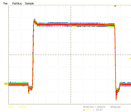
Figure 5 Switching Node (10V per Division)
