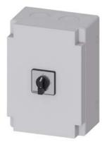
SENTRON, Switch disconnector 3LD, change-over switch, 3-pole, lu: 100 A, Operating power / at AC-23 A at 400 V: 37 kW, molded-plastic encapsulation for metric cable screw connection, knob-operated mechanism, black
