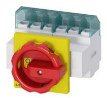
SENTRON, Switch disconnector 3LD, emergency switching-off switch, 6- pole, lu: 32 A, operating power / at AC-23 A 400 V: 11.5 kW, front-mounted, rotary operating mechanism, Red / yellow, 4-hole mounting of the handle
