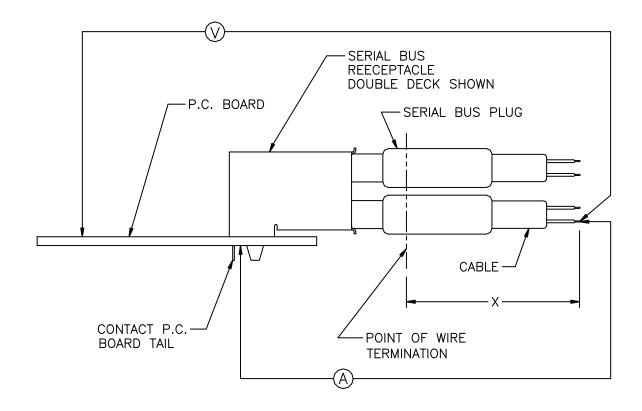
1.RESISTANCE DUE TO X INCHES OF IS TO BE REMOVED FROM ALL READINGS FIGURE 1
