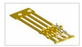
Leadframe Type: Single-In-Line (SIL) Centerline (Pitch): 2.54 mm [ .1 in ] PCB Thickness (Accepted): 1.6 mm [ .063 in ] Standoff Height: 1.7 mm [ .067 in ] Leadframe Hold-Down Feature: Without
