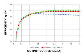
Figure 7. Converter Efficiency versus Output Current.
