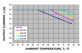
Figure 8. Derating Output Current versus Ambient Temperature and Airflow.,  $V_{\rm IN}$ =12V
