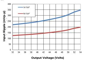
Figure 25. Input ripple voltage. Input voltage is 12V. Scope BW
