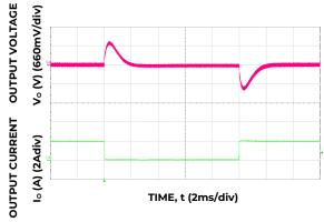
Figure 4. Transient Response to Dynamic Load Change from 50% to 0% at 12V $_{\text{in}}$ ,  $C_{\text{out}}$ =3x10uF+470uF,  $C_{\text{Tune}}$ =1000pF, R<sub>Tune</sub>=30.1kΩ
