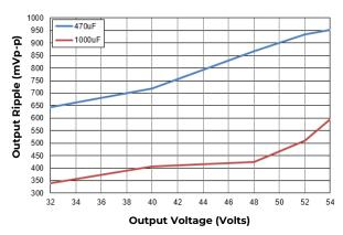
Figure 26. Output ripple voltage .Input voltage is 12V.
