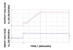
Figure 24. Typical Start-up Using Input Voltage (V  $_{\text{IN}}$  = 12V,  $_{\text{I}_{\text{O}}}$  =  $_{\text{I}_{\text{O},\text{max}}}$ ).
