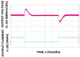
Figure 16. Transient Response to Dynamic Load Change from 50% to 0% at  $12V_{in}$ ,  $C_{out}$ =470uF,  $C_{Tune}$ =1000pF,  $R_{Tune}$ =30.1k $\Omega$
