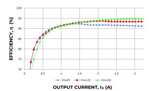
Figure 13. Converter Efficiency versus Output Current.
