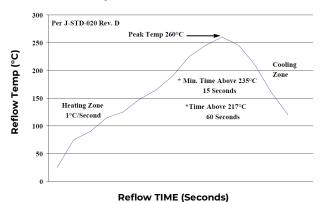
Figure 35. Recommended linear reflow profile using Sn/Ag/Cu solder.
