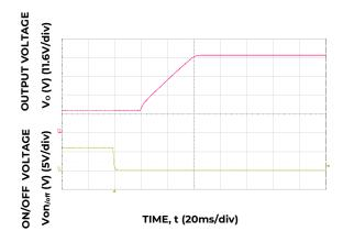
Figure 17. Typical Start-up Using On/Off Voltage ( $I_0 = I_{0,max}$ ).
