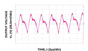
Figure 3. Typical output ripple and noise ( $C_0=3x10uF+470uF$ ,  $V_{IN}=12V$ ,  $I_o = I_{o,max}$ , ).
