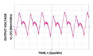
Figure 15. Typical output ripple and noise(Co=3x10uF+470uF,  $V_{IN}$  = 12V,  $I_o$  = I  $_{o,max_7}$  ).
