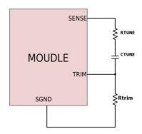
Figure. 31. Circuit diagram showing connection of  $R_{\text{TUME}}$  and  $C_{\text{TUNE}}$  to tune the control loop of the module
