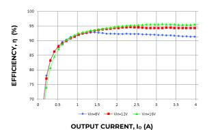
Figure 1. Converter Efficiency versus Output Current.
