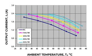
Figure 20. Derating Output Current versus Ambient Temperature and Airflow. V<sub>IN</sub> = 14V
