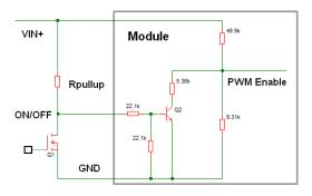
Figure 27. Circuit configuration for using negative On/Off logic.
