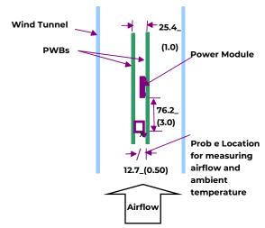
Figure 32. Thermal Test Setup
