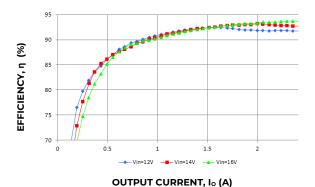
Figure 19. Converter Efficiency versus Output Current.
