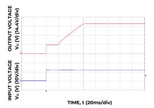
Figure 18. Typical Start-up Using Input Voltage (V  $_{\mbox{\scriptsize IN}}$  = 12V,  $_{\mbox{\scriptsize Io}}$  =  $_{\mbox{\scriptsize Io},max}$ ).
