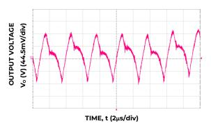
Figure 9. Typical output ripple and noise ( $C_0=3x10uF+470uF$ ,  $V_{IN}=12V$ ,  $I_0=I_{o,max}$ , ).
