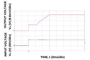
Figure 6. Typical Start-up Using Input Voltage (V<sub>IN</sub> = 12V,  $I_o = I_{o,max}$ ).
