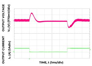
Figure 22. Transient Response to Dynamic Load Change from 50% to 0% at  $12V_{in}$ ,  $C_{out}$ =470uF,  $C_{Tune}$ =1000pF,  $R_{Tune}$ =30.1k $\Omega$
