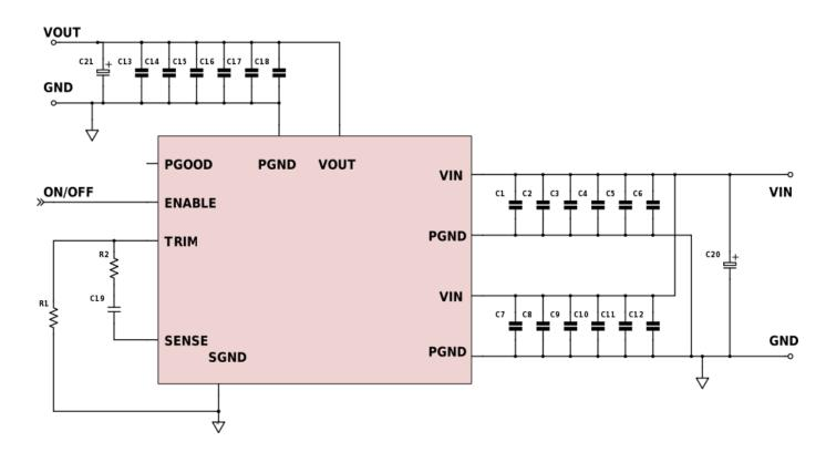
C2-C6, C8-C12 4.7µF/25V, 1210 ceramic capacitor C1,C7 0.047uF/50V,0603 ceramic capacitor
