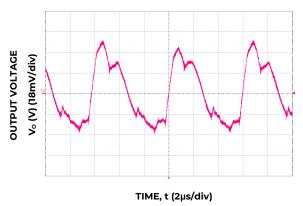
Figure 21. Typical output ripple and noise  $(C_0=3x10uF+470uF, V_{IN}=12V, I_0=I_{o,max})$ .
