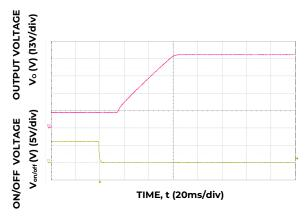
Figure 23. Typical Start-up Using On/Off Voltage  $(I_0 = I_{0,max})$ .
