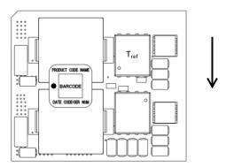
Figure 32. Preferred airflow direction and location of hot-spot of the module (T<sub>ref</sub>).
