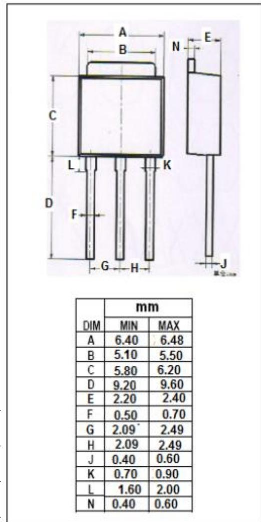
**isc N-Channel MOSFET Transistor****IRLU120N****ELECTRICAL CHARACTERISTICS** $T_C=25^{\circ}\text{C}$  unless otherwise specified
