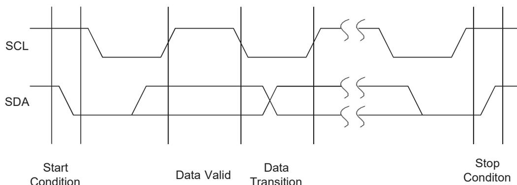
Figure2: Timing diagram for output ACKNOWLEDGE
